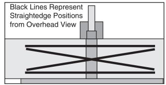
**Figure 50.** Straightedge positions for checking infeed/outfeed table parallelism.
